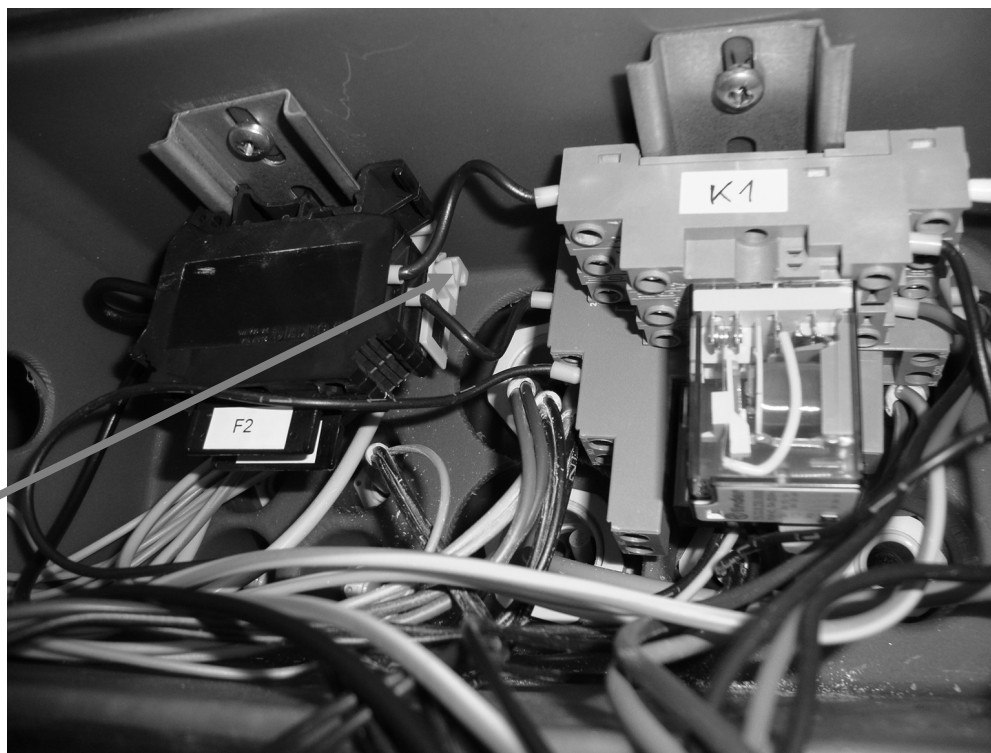
Fig. D-2: Position of protective grounding conductor terminal
