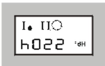
The raw water hardness stored in the system is displayed. You must now enter the actual raw water hardness applying at your installation site. You can determine this value by means of the "Total hardness" water analysis kit or by inquiring at your local water works.
