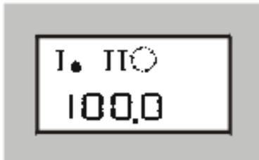
The water meter pulse just set is displayed (l/pulse).
