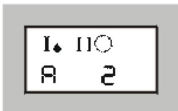
A 2 is displayed for a system with two exchanger tanks. The code for a system with one exchanger tank is A 1. The setting must be changed as required.
