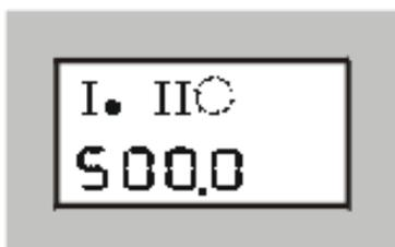
The nominal capacity stored in the record is displayed. This setting cannot be modified.
