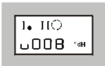
The "blending hardness" menu item is displayed. Enter 0 °Gh if your system does not have a blending unit at all or if the blending unit is installed before the water meter. In all other cases, the blending hardness value must be set. The value is determined by the setting of the blending valve (between 0 °Gh and the raw water hardness). If drinking water is to be softened, the guidelines set out in the German Drinking Water Act must be complied with (refer to section E).
