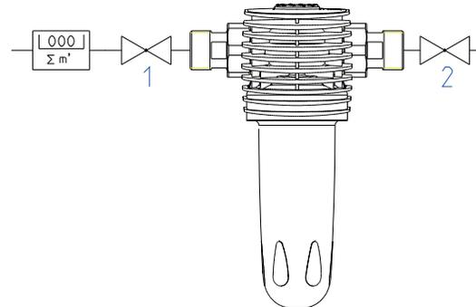
Fig. 1: Installation drawing BOXER® K front view
