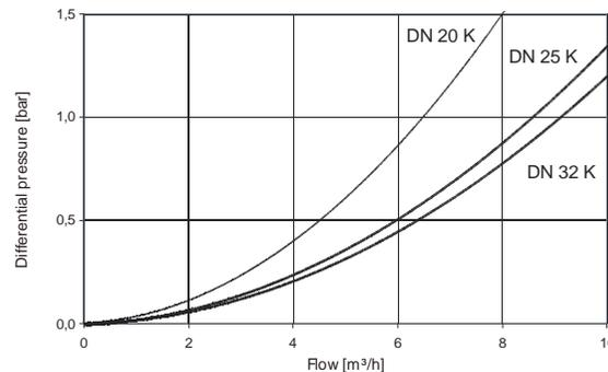
Fig. 3: Pressure loss curve K and KD
