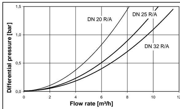
Fig. 5: Pressure loss curve BOXER® R / A
