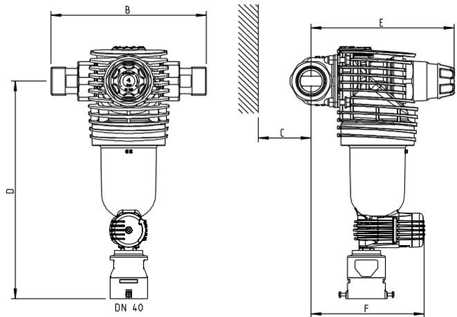
Fig. 4: Installation example backwash filter BOXER® RD
