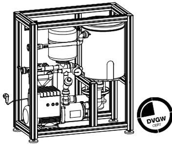
Fig. 1: Euro-system separation device GENO®-G5
