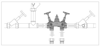
Installation example with water meter screw connection
