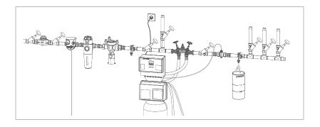
Measure the blending hardness using the water test kit at the sampling tap.
