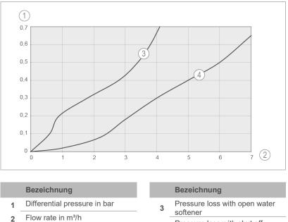
4 Pressure loss with shut off water softener
