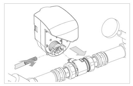
3. Place the protectliQ onto the ball valve.
