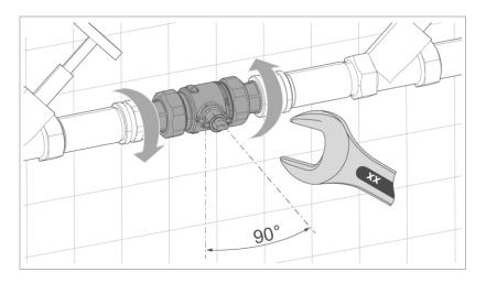
**6.** Tighten the ball valve with the union nuts without applying mechanical stress.
