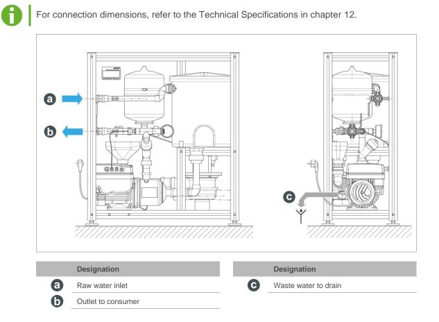
A drain connection (at least DN 50) must be available, which is able to discharge the maximum inlet volume in the event of a malfunction.
