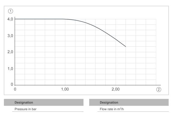
Note: Valid with built-in flow restrictor in the water outlet (as delivered)
