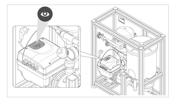
The operating panel of the pressure booster system indicates the system status and outputs error messages.
