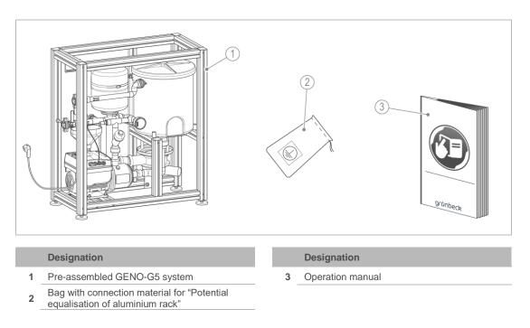
• Check the scope of supply for completeness and damage.
