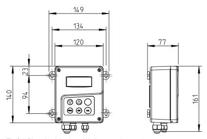
Fig. C-1: Dimensional drawing - pH/redox measuring transducer
