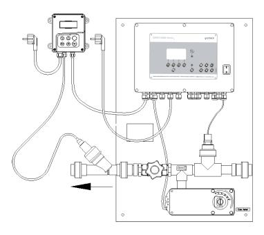
Fig. D-2: pH value or redox monitoring equipment installation example mounted on GENO-KWA50k
