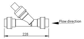
Fig. C-2: Dimensional drawing - pH/redox measuring point DN 25
