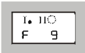
The parameter "Water Meter Pulse" is displayed. Table F-1 indicates what the codes represent.
