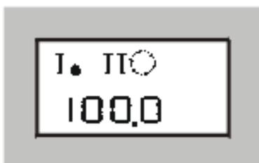
The water meter pulse just set is displayed (l/pulse).
