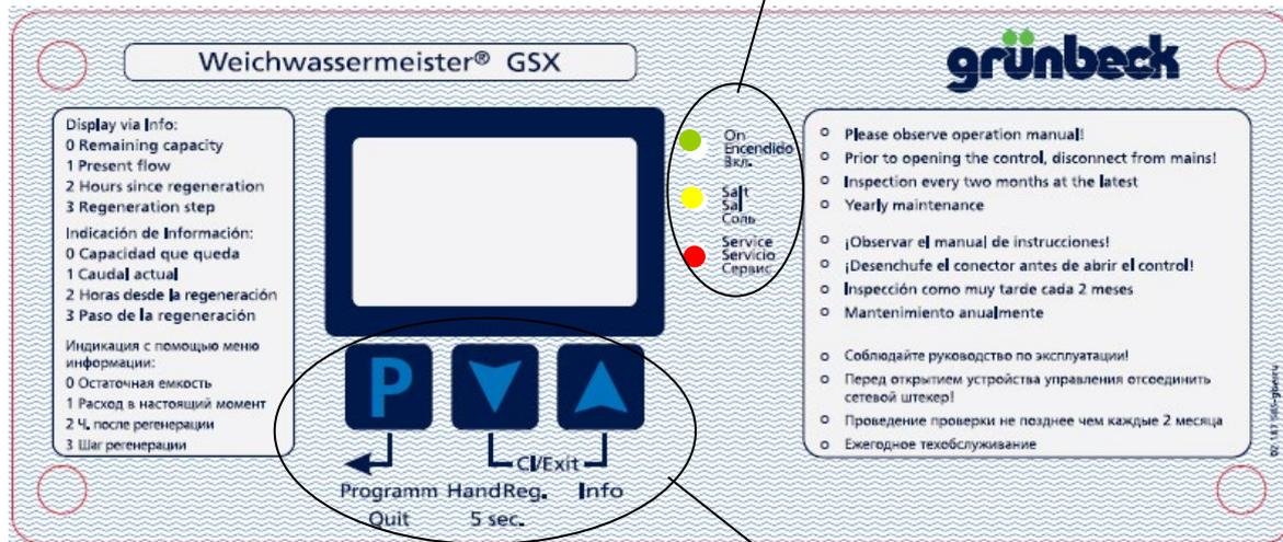
Fig. F-1: Operating panel of Weichwassermeister GSX Operating keys
