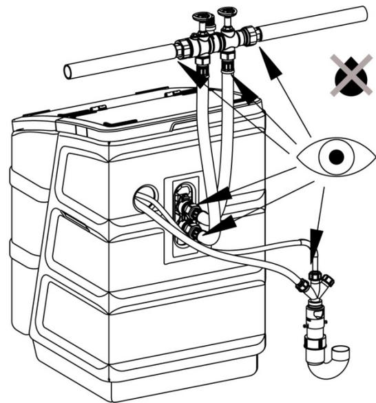
2. Visually check for tightness (check at the connection block as well).
