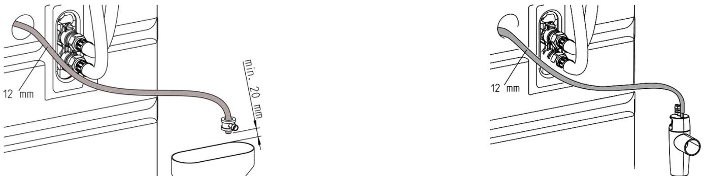
Fig. D-3: Drain connection of rinsing water hose with and without accessory drain connection DN 50 according to DIN EN 1717 (order no. 188 875)
