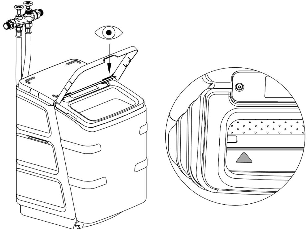
Fig. H-2: Marking line at brine tank funnel
