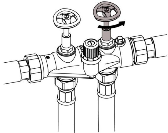
6. Open the shut-off valve for soft water at the connection block.
