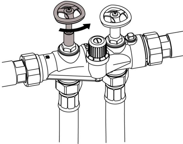
1. Open the shut-off valve for raw water at the connection block.
