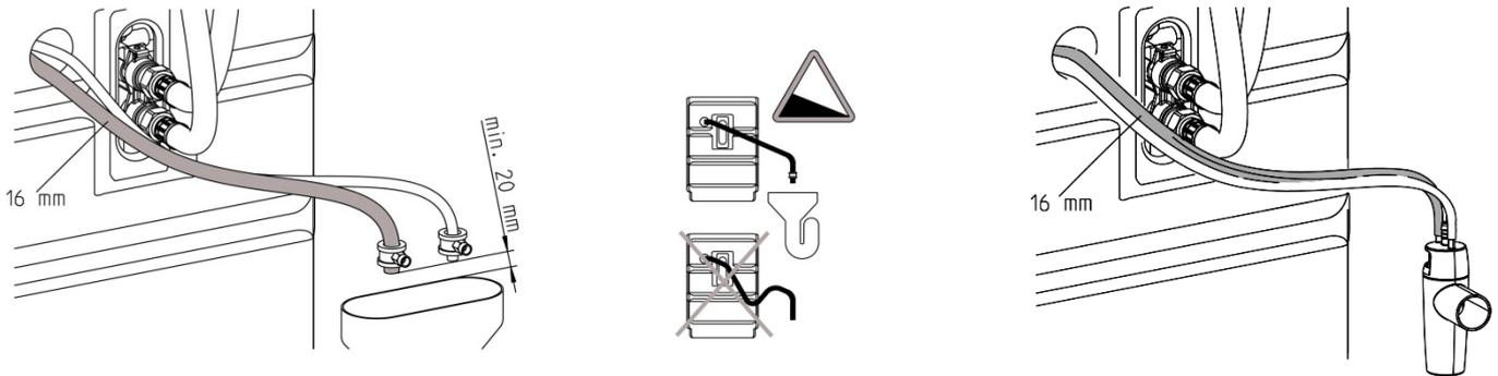
Fig. D-4: Drain connection of overflow hose of brine tank with and without accessory drain connection DN 50 according to DIN EN 1717 (order no. 188 875)
