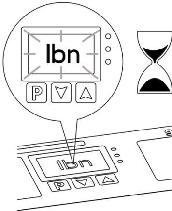
5. During system deaeration, "lbn" is indicated in the display and after approx. 6 minutes into the subsequent twin regeneration, the time is displayed.
