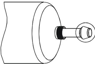
Fig. C-2: Quartz protective pipe GENO UV-200 S
