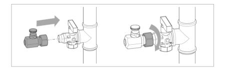
**4.** Connect the KFE boiler fill and drain fitting to the KFE boiler fill and drain shut-off valve of the heating system.
