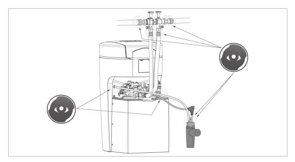
14. Visually check the connection points for leaks.
