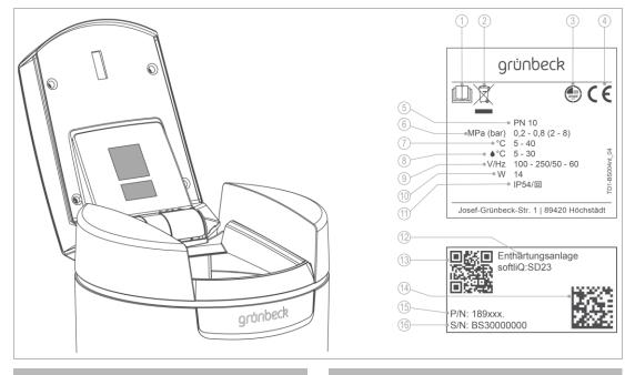
The type plate is located on the inside of the brine tank lid.
