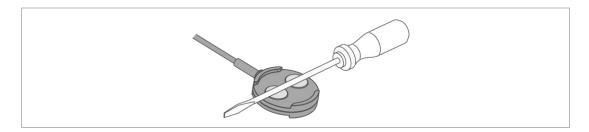
» The water sensor is working if the water softener issues a warning message after 30 seconds at the latest.
