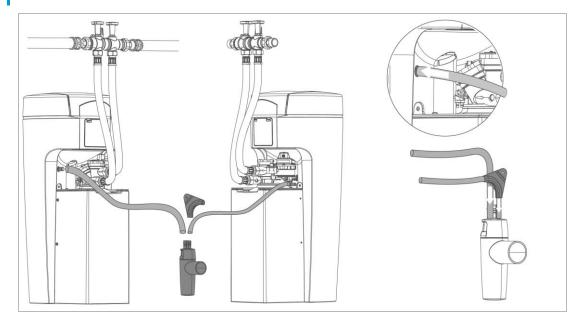
1. Shorten the flushing water hose (Ø 12 mm) to the required length.
