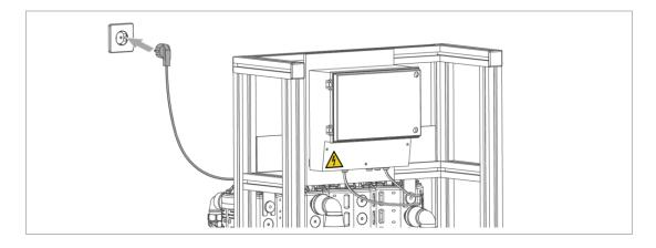
▶ Plug the mains plug into the 230 V socket.
