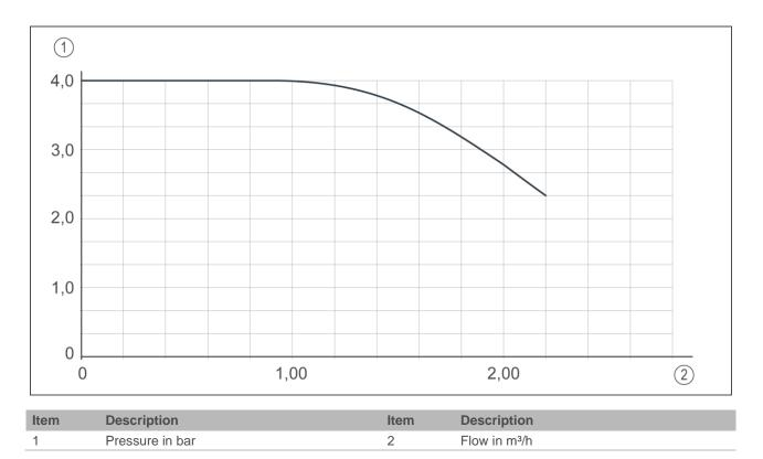
Note: Valid with built-in flow restrictor in the water outlet (as delivered)
